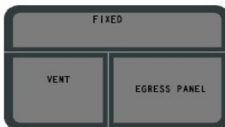
F300SVSE (F300SESV OPPOSITE) MINIMUM 36 1/6 X 30 1/8 MAXIMUM 72 X 48 AT 51 7/8 WIDE & OVER IT BECOMES EQUAL SIDED
